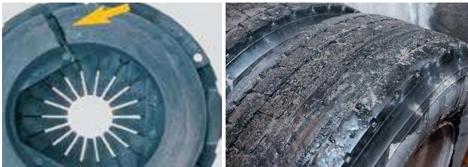
Figure 2 Fracture and overheating of the pressure disc with constant slippage of the clutch
